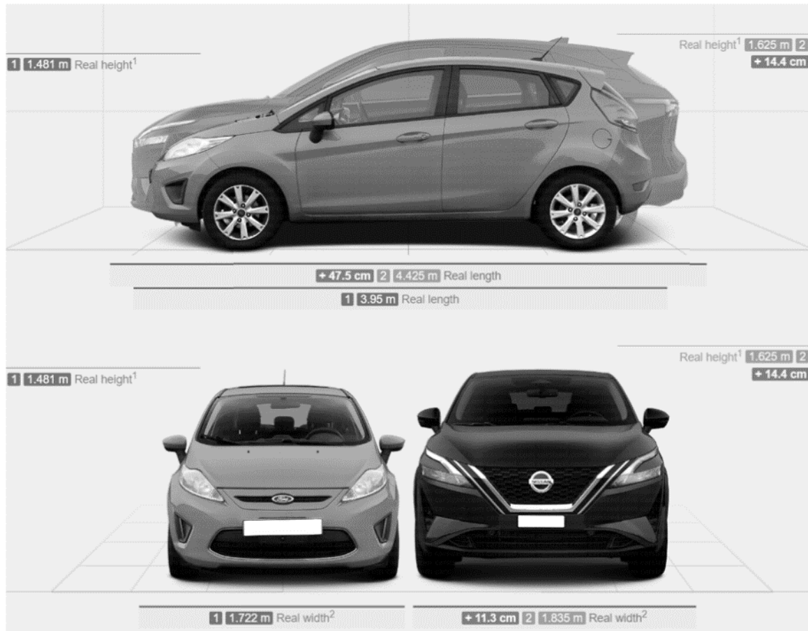
Figure 1. Ford Fiesta (JA8) 5-door Hatchback 2008 compared with Nissan Qashqai (J12) SUV 2021 (carsized, 2023).
