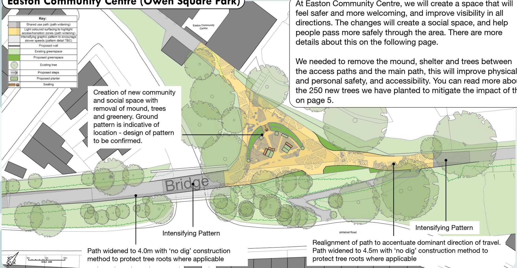
Path widened to 4.0m with 'no dig' construction method to protect tree roots where applicable
