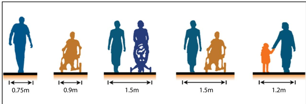
Figure 4: Typical widths required by pedestrians and wheelchair users<sup>7</sup>
