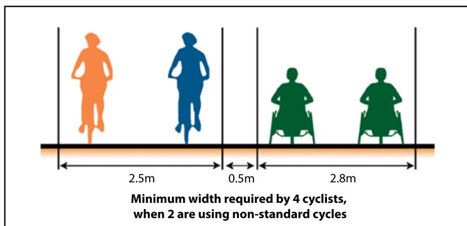
Figure 3: Widths for wider cycles, including non-standard cycles<sup>6</sup>
