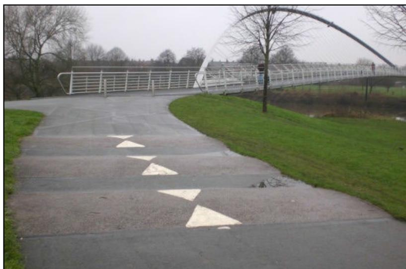
Figure 9: Speed humps on cycle track, York
