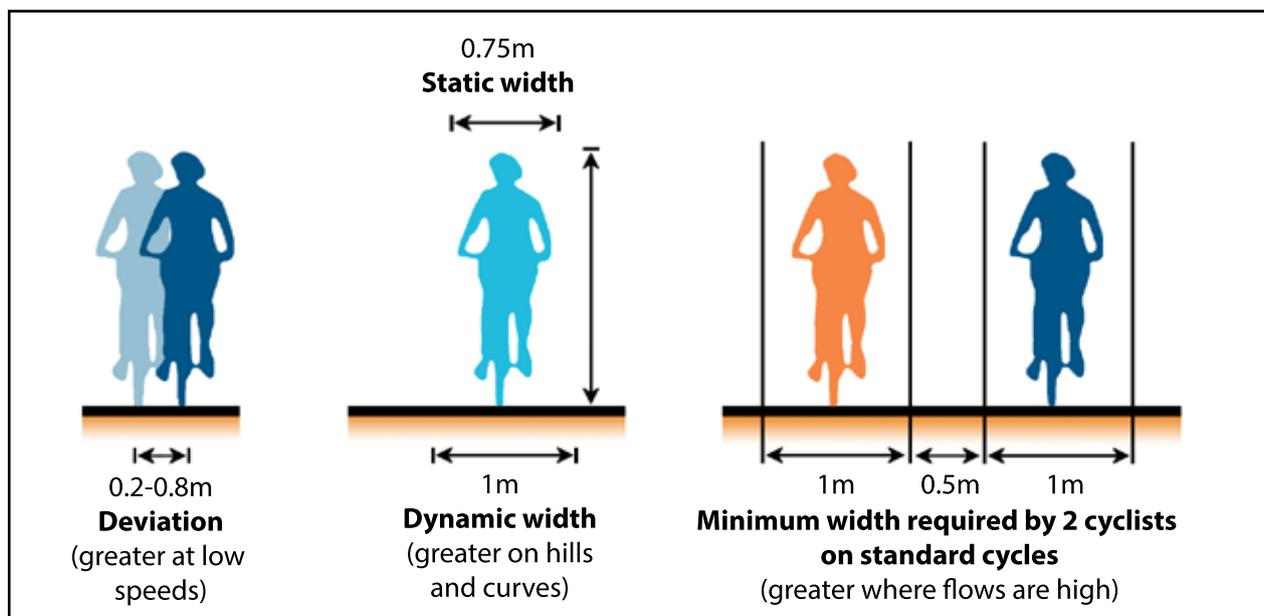
Figure 2: Required and dynamic widths for cycles<sup>6</sup>
