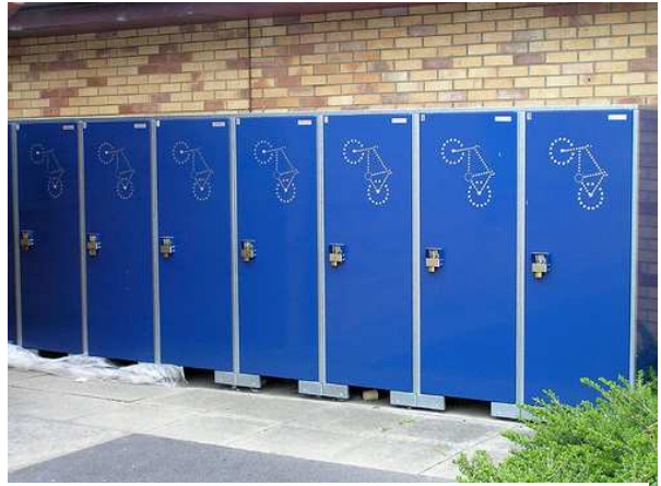
Bike lockers can be a secure and space efficient form of storage
