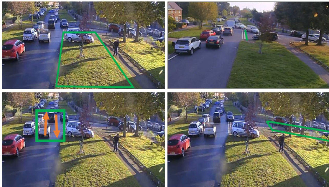
Figure 18: Markings for behaviours at Hillstone Video Location 1. Parking on grass verge (top left), interactions between drivers within junction area (bottom left), drivers manoeuvring over give way lines (top right), and parking in School Street (bottom right).
