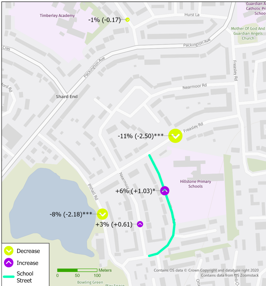
Figure 14: % (and numerical) change in average morning traffic speeds (08:00-09:00) between baseline and follow-up
